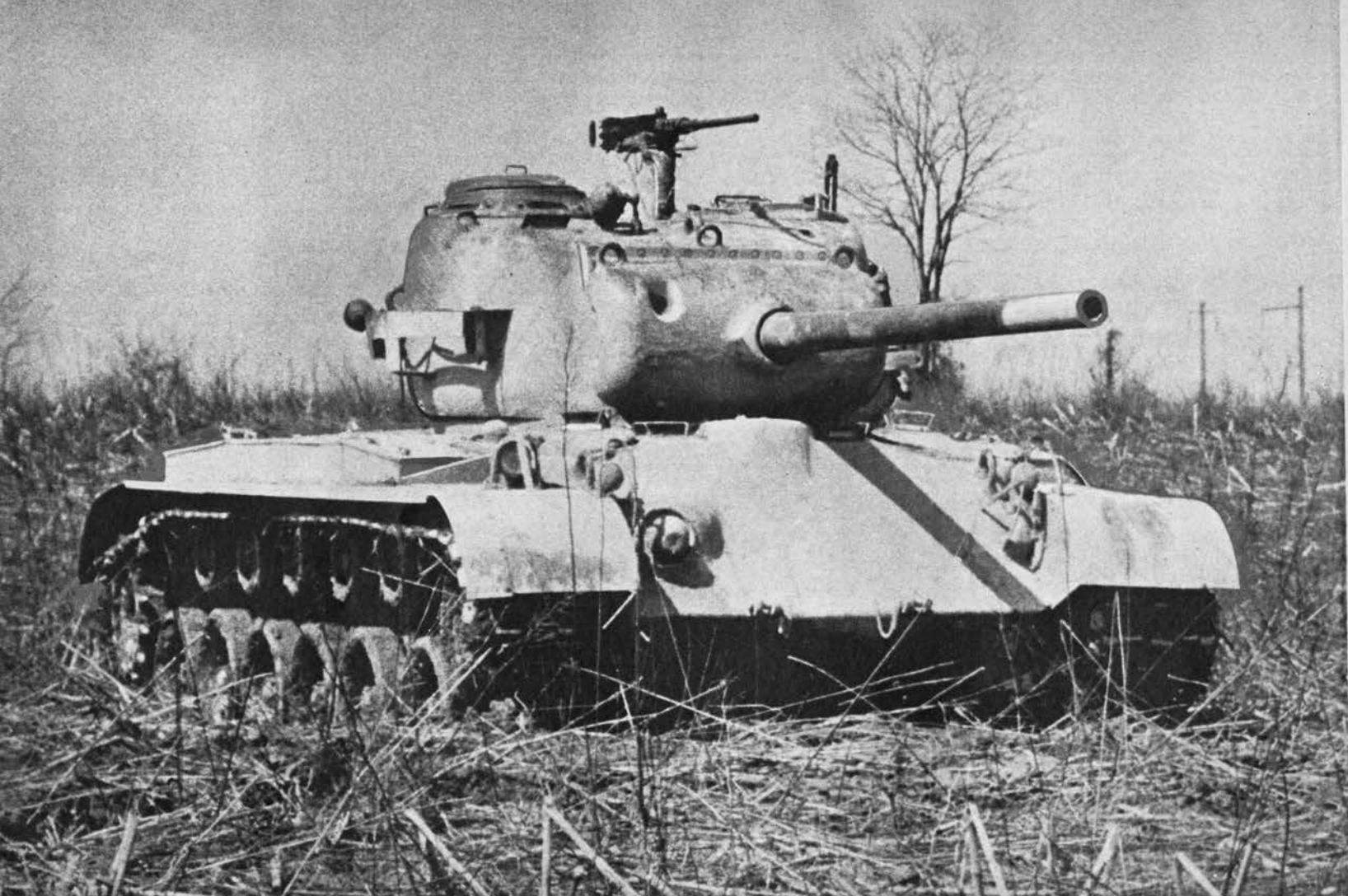
HUGE TURRET, SQUAT CHASSIS OF M-26 GIVE IMPRESSION OF GREAT POWER. BIG 90-MM. CANNON PROTRUDES SEVERAL FEET BEYOND TANK'S BOW
